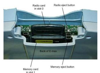
E-max will auto-detect the insertion of the card and automatically locate a valid EGC network and identify itself to the network.
