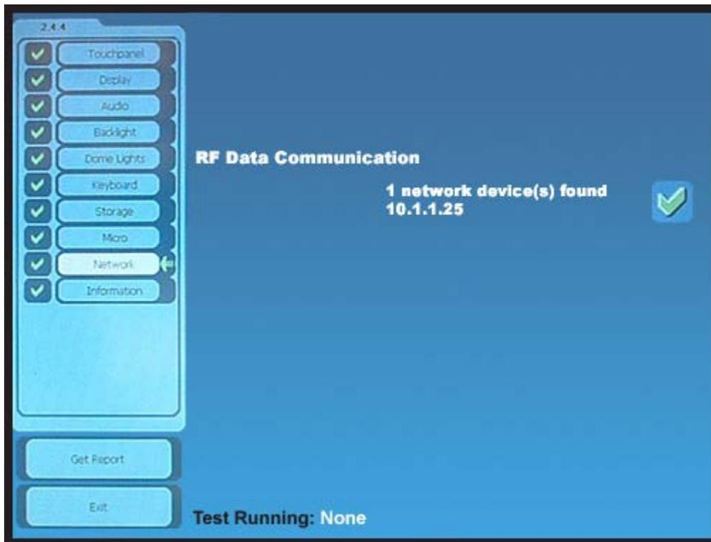
Searches for a valid EGC RF or Ethernet network and then displays the information of the network found or indicates if no network could be found.
