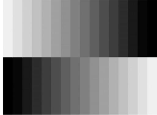
**NOTE:** Small variations in the absolute shade of each color are normal. Depending on the age of the unit, a few pixels may no longer be active, or the backlight may become slightly dimmer. The unit can still be used for gaming. However, if the display image is inadequate for player use during gaming, or fails the test, the unit requires EGC Factory repair.
